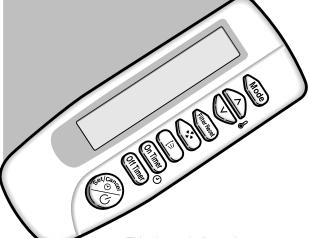
This chapter indicates how to operate and program your air conditioner with the wireless remote controller. The wireless remote controller is an optional accessory.
